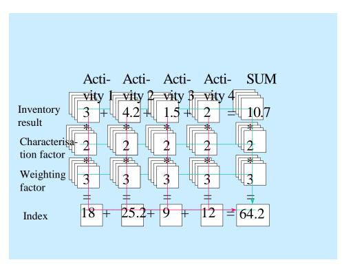
Figure 3.1 LCA by EPS (first vertical and then horizontal) compared to conventional LCA (first horizontal and then vertical)
