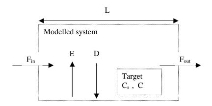
Figure 4.2 Modelling of a characterisation factor with the *empirical method*  $F_{in}$  and  $F_{out}$  are the mass transport of the modelled substance in and out of the system, E and D the emission and deposition within the system and C<sub>s</sub> and C the system related and total exposure concentrations at the target.
